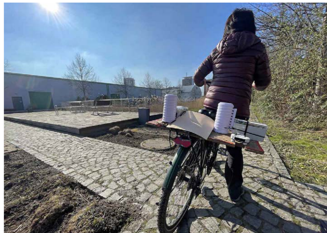
Citizen scientists collect climate data using a bike-mounted sensor. The climate data is uploaded to the open-source platform sensemap. CityCLIM CS project. Photo: Peter Barczewski/3d-artstudio
